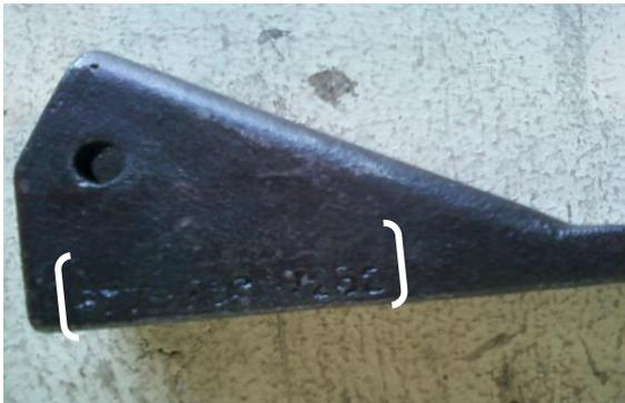
This is a close up of the phone number on the side. If you hit the phone number the tips should be replaced as soon as possible.
