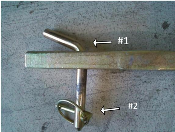
This is the pin that holds the Shank to the TR3 or Rascal. The main pin #1 is a bent pin and the second pin #2 is a lynch pin.
