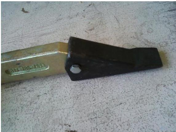
This is the tip bolted on to the Shank. The standard Shank on a TR3 or Rascal is a 9" shank.
