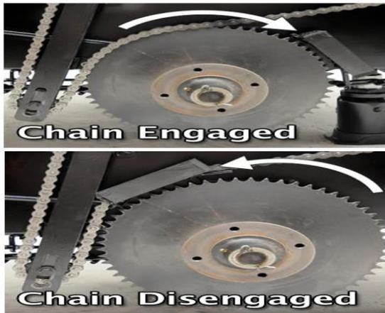
The operating lever labeled #2 in the above photo controls the chain engagement mechanism. This allows the chain to be disengaged and engaged one tooth at a time and helps keep the chain and sprocket in alignment. This also helps reduce unneeded repair, wear and tear, and breakage.
