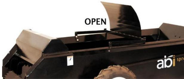
The optional end gate is used to prevent manure from spilling out during filling or transportation, and to help further deflect material from the operator during spreading. The end gate should never be down when spreader is in use. For models 25 – 50 the end gate must be operated manually. For larger models 85 – 130 there is an optional hydraulic lift arm. Having this down during use may cause damage to the hood or tool.
