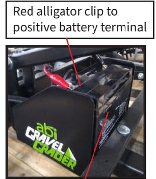
Fig 9. Red alligator clip to positive battery terminal
