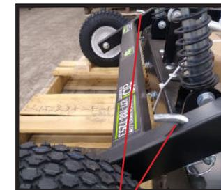
Fig 11. Bent Pins w/ Lynch Pins storage positions
