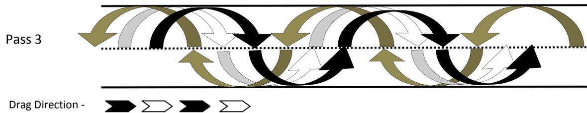
The white arrows indicate the first pass. The gold arrows are the second, and the black arrows the third. You will come down the drive in the same slow serpentine pattern, then starting at the bottom repeat the pattern, continuing up and down; till the waves are fully removed.
