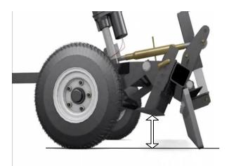
Grading with the Finish Rake: You can use the finish rake like a grading blade. For this lower the wheel down, and either flip the profile blade or scarifiers over to the top, or raise them so they can not touch the footing. Lower the finish rake down so that it is close to a 90 degree angle, and then you are ready to grade. This is useful for moving large amounts of dirt or footing, or repairing footing in an arena.
