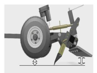
To set the Depth: Place the Rascal on a hard surface. Raise the finish rake up so the Rascal will set on the scarifiers and wheels. Then raise the wheels up to about the depth you wish to drag. Example – if you want 2" of ripping depth set the distance from the bottom of the wheel to the ground around 1  $\frac{1}{2}$ " from the surface. Mark this on the shaft of the actuator or the hand jack to ensure hitting the same mark later.
